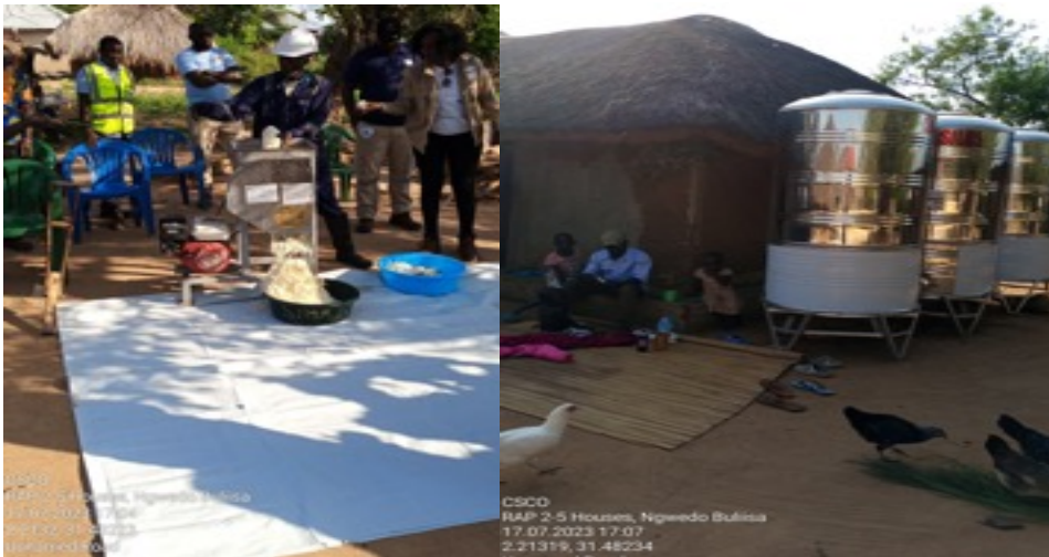
Figure 20: Some of the technologies such as (left) cassava chipper for processing cassava, (right) cassava silos for storage of the processed cassava, introduced to the PAPs and project affected community
